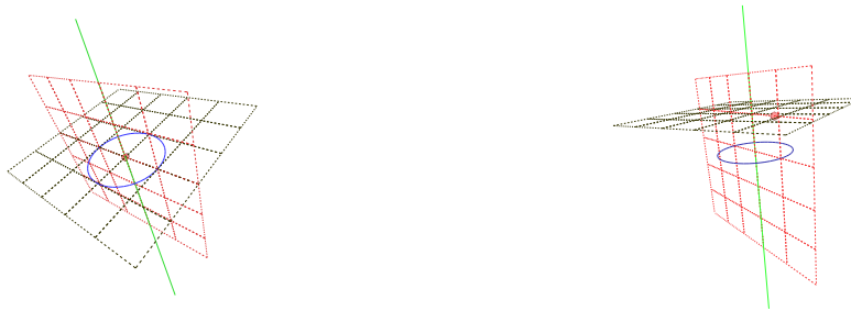
Figure 5.6: A Circle (in blue) and Line (in green) are contracted with a Flat Point (the small red sphere) to create a red plane orthogonal to the circle and a yellow plane orthogonal to the line.
